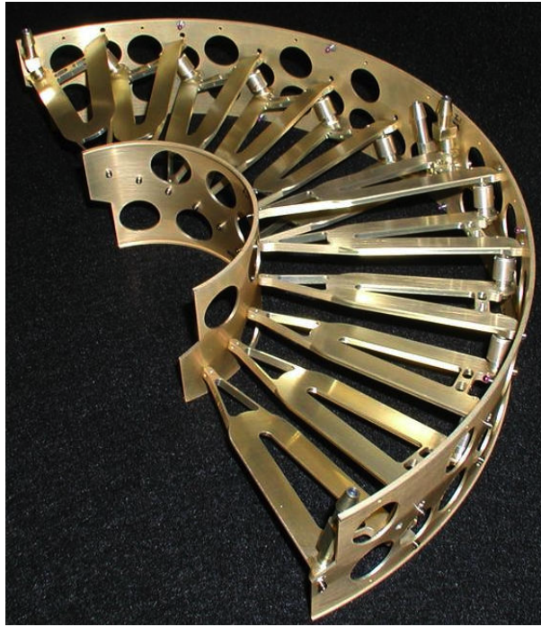
Figure 2.13: The FPix half-disk cooling channels mounted in the outer half-ring structure. The turbine-like geometry is apparent. Panels are mounted on both sides of the cooling channels [20].
