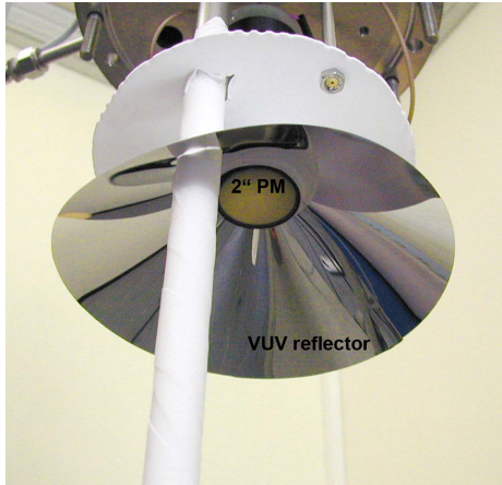
Figure 5: Inside the vessel. The geometry used for the measurements with the phototube, pointing downwards.
