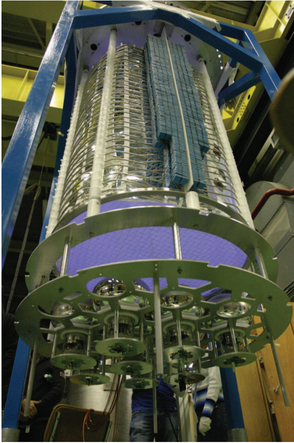
Fig. 5: The light readout installed in the ArDM experiment and illuminated with an UV light (254 nm).
